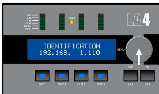
Figure 19: Launching the Identification function
