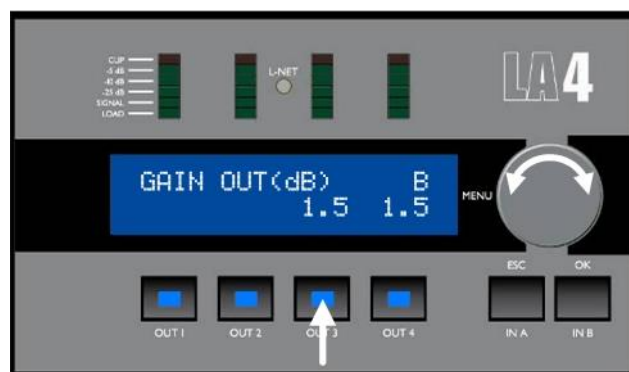
Figure 17: Setting the OUT 3 gain
