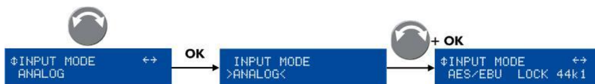
Figure 30: Selecting the input mode
