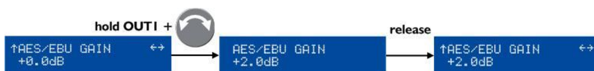
Figure 35: Setting the AES/EBU GAIN
